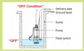
Built-in float switch for 1 Phase pumps to prevent dry run of motor.
